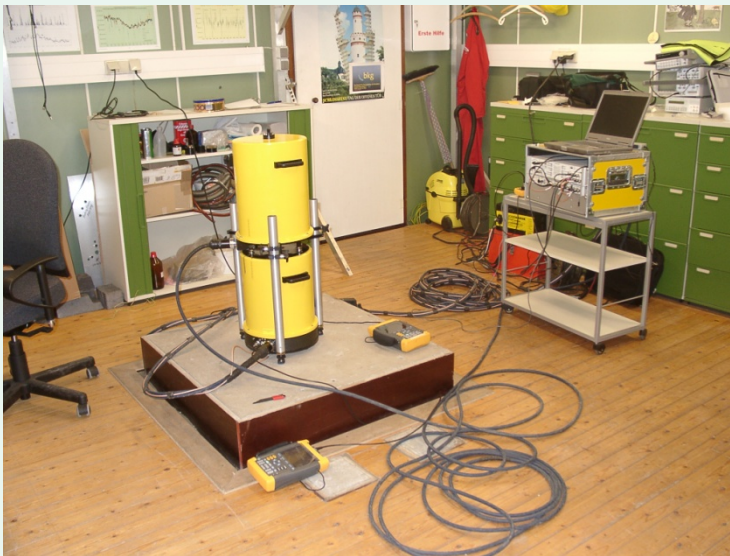
A10 reference measurement at Bad Homburg station
