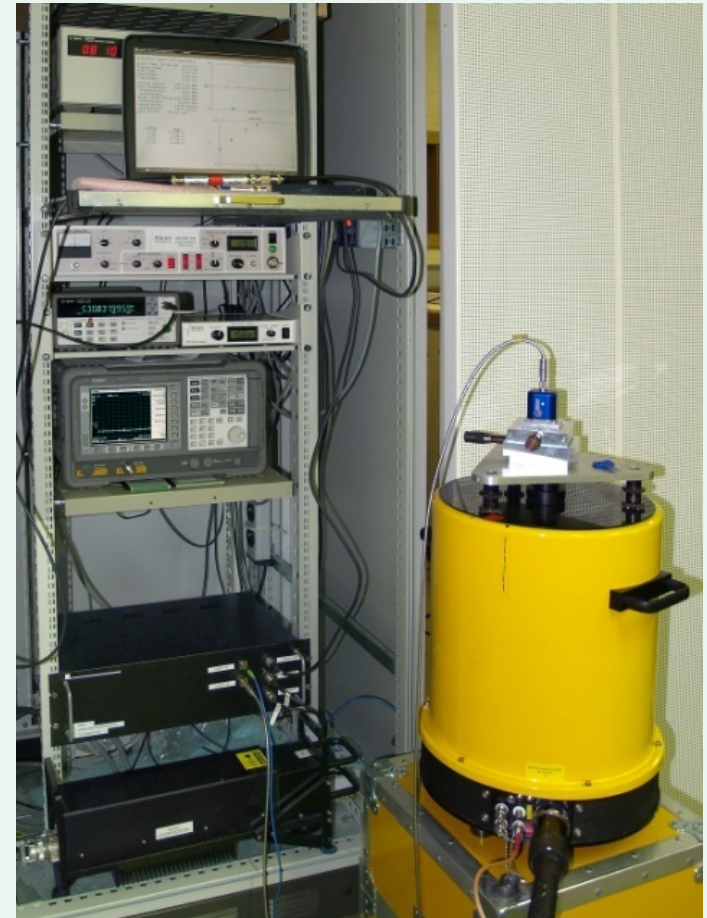
A10 check with laser heterodyne and cesium standard
