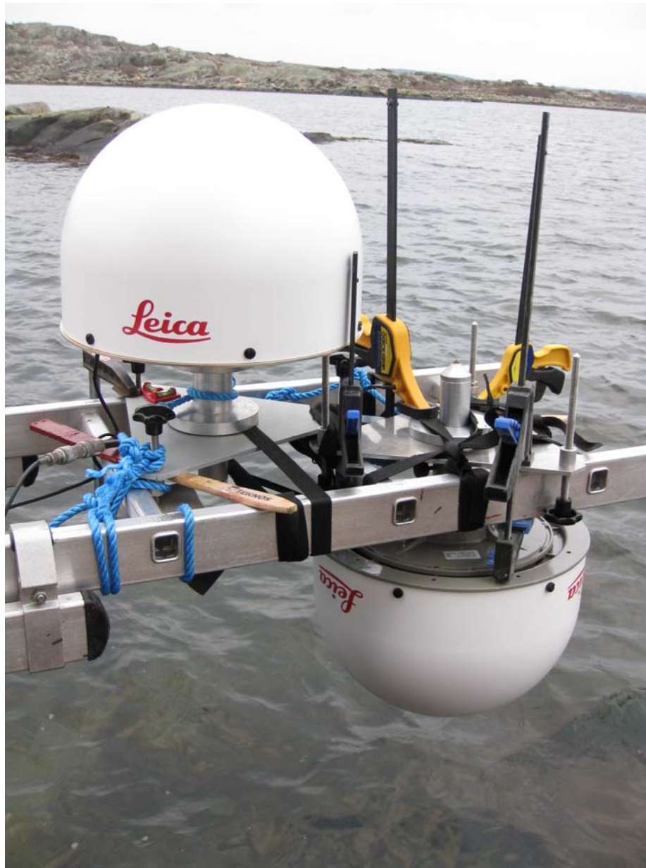
Right-circular polarised antenna
